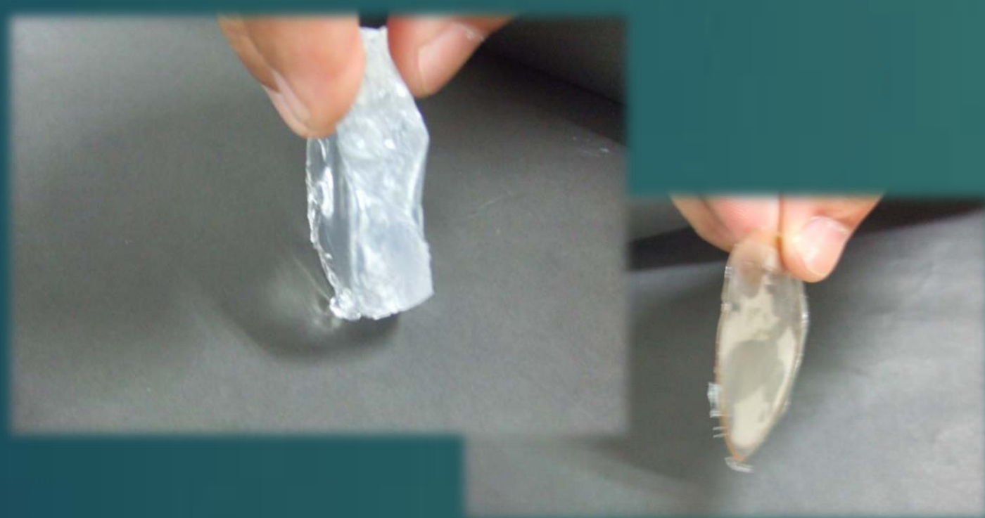
Poly(vinyl alcohol)/chitosan hydrogel, swollen and dry states, was used in this study
